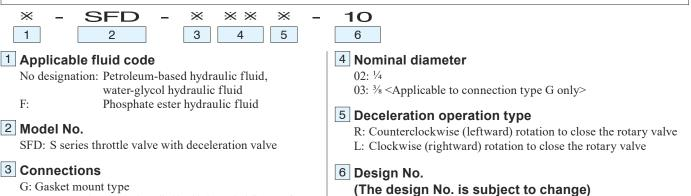
T: Screw connection type <Only applicable with the nominal diameter of "02">
